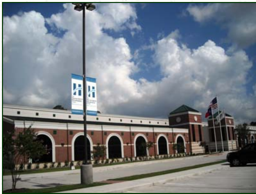
POLE BANNERS ARE DOUBLE SIDED 6'X2' HEAVY DUTY VINYL, SECURED ON TOP AND BOTTOM
